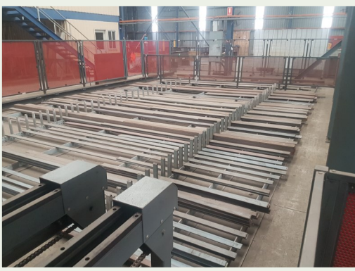
Flat Bar storage area with infed system
